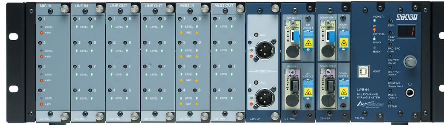
LWB-64 with MIC IN, LINE IN, LINE OUT, AES3 IN, AES3 OUT and 2-wire INTERCOM modules (video transmission modules and converters are optional)
